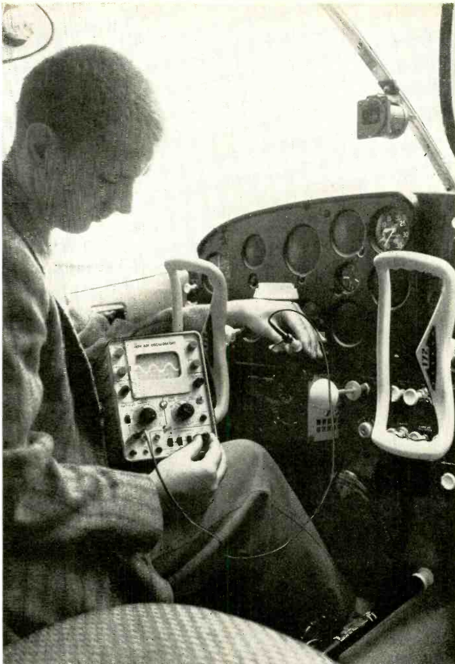
Because it has its own power supply, the scope may be used in servicing small-plane equipment.
