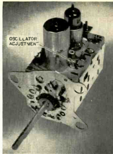
Fig. 11 — Tuner in G-E's M6 chassis. The oscillator trimmer is near the output jack.
