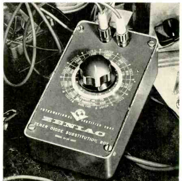
Zeniack, a 10-watt Zener diode substitution box made by International Rectifier.
